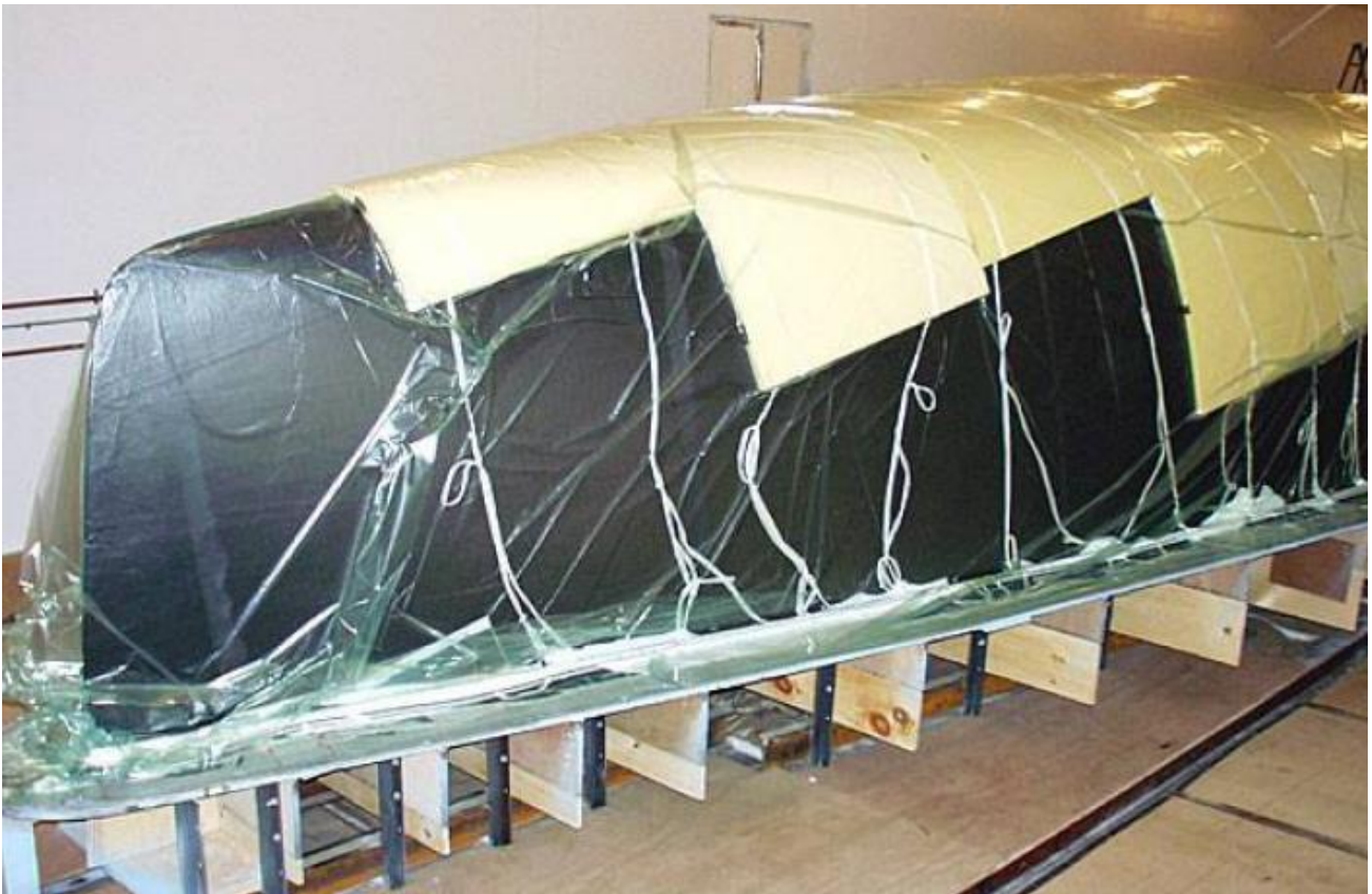
Figure 1 - Thermo-forming core over a male moulded yacht hull
