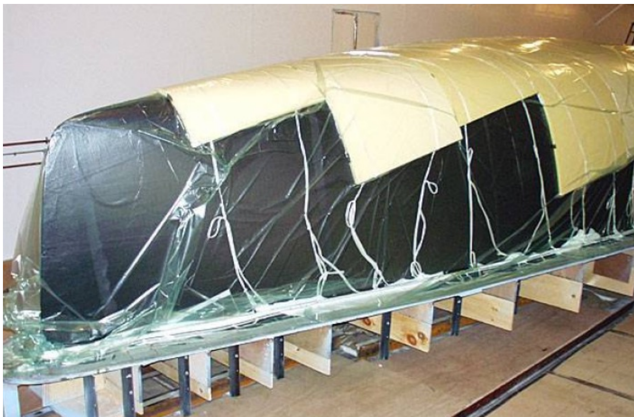
Figure 1 - Thermo-forming core over a male moulded yacht hull
