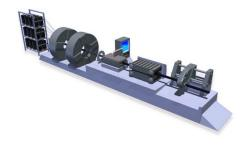
In pullwinding process the fibers are impregnated with a thermoset resin and pulled through a heated die where curing takes place.
