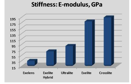
**PULLWINDING** process enables the reduction of wall thickness and weight while retaining and improving stiffness and strength compared to conventional pultrusion.
